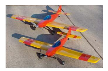
The new model, which I named the Fusion 380, has a measured RTF weight of 40.6 oz. I was able to come very close to the target weight and both planes fly in a similar manner and with the same perceived "feel".
