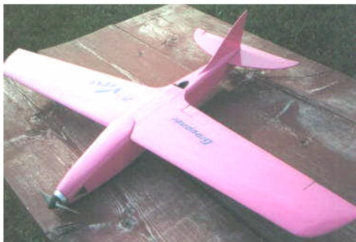
SP400 6V motor, APC 4.75x4.75 prop, 7 x 500AR cells, Viper MD102 ESC, Hitec 535 RX with Maxx Products MX-50 servos, flying weight about 17 oz. An excellent Graupner kit that's easy to build. It's not really competitive with the current crop of pylon racers, but it makes a great sport plane that's not a handful to launch and land and is rugged enough for rough fields. Plenty of room inside for the radio gear and battery. Unique
