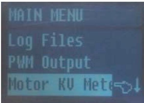
Once the Motor KV Meter is highlighted, **tap** the bottom (Menu) button and the KV Meter screen opens. It may or may not have the correct number of Poles (magnets) in the upper right corner.
