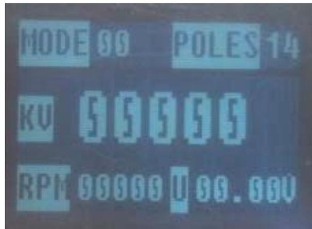
The Motor KV Meter was ready to be used, and in this case, with logging turned on. **Unfortunately, logging cannot be used when the Motor KV Meter is in use.** Logging may only be initiated when one of the five monitors is in use. A lesson learned.
