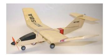
(1) POLY-T (is a construction article in the November 2006 RC MICRO WORLD online magazine [http://www.cloud9rc.com]). It is 110 square inches and weighs only 4.6 ounces with a Bob Selman Mighty Midget Gold Series 13/4/15T brushless outrunner (weighs 7 grams) and two 300mAh Li-Poly batteries. The plane was designed to resemble a small commuter liner.
