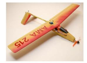
(2) EAGLET-II (will be in the January 2007 RC MICRO WORLD). It is 75 square inches and weighs 5.4 ounces with a Feigao brushless inner runner running a GWS 3x3 pro direct on two 340 mAh Li-Poly cells. This little plane features a flat 3/16 balsa wing (no airfoil) with a hardwood dowel leading edge. The tail boom is a Sports Authority carbon fiber arrow shaft. The inverted "V" tail is just to be different.
