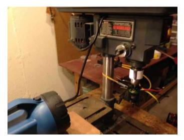
The photo shows a drill press set up to measure its RPM. A white band of paper was placed on the drill press chuck with two vertical black lines marked on the paper 180 degrees apart. To operate correctly, an optical tachometer requires either natural or DC generated light. Standard AC house lighting will not work. The flashlight provides the DC light source for using an optical tachometer when the AC lights are shut off.
