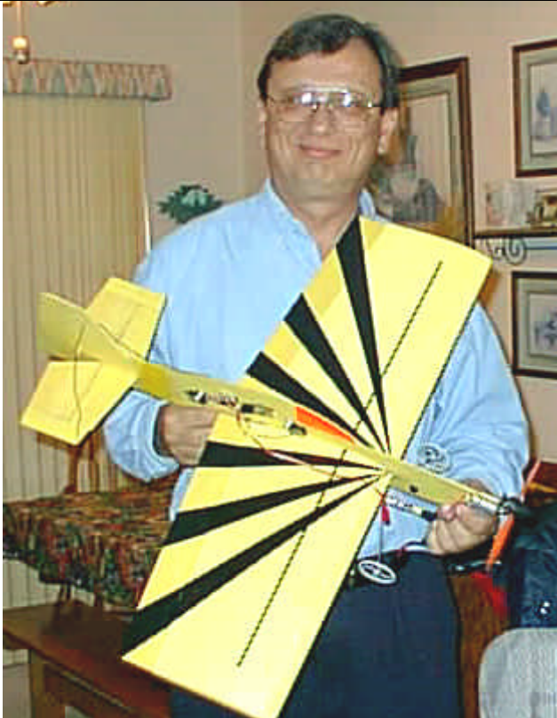
The Sopwith Pup is Jack Lemon's and produced by, Kavan. It is all foam. Jack had to pre-wire everything and then stuff it in. It weighs 18.4 ounces.
