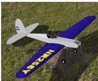
The photo shows my Race-E, built from the free pullout plan in the February 2005 *Fly RC* magazine. The AXI 2208-26 using a 7x4 prop powers it. It weighs 10 ounces and is finished with the silver/gray and blue of the Hughes H1.
