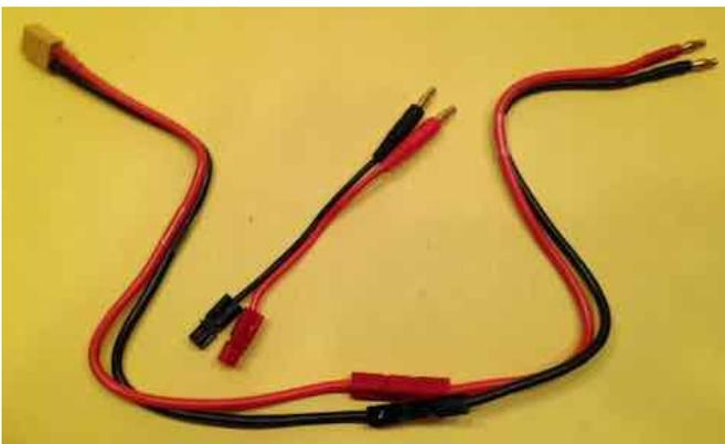
I clipped the DC Input Power Cable in half and added Anderson Power Poles (APPs) to the clipped ends. I use APP connectors on my alligator clips from my Marine/RV battery to the charger. If another power supply is ever used with this charger, I wanted to keep the banana plug option available.
