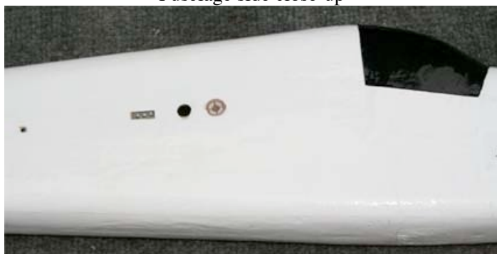
Fuselage side showing the socket for the locator pin aft.
