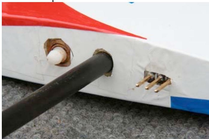
Wing root. The socket for the ball/stick was made from a wood dowel rather than the plastic one supplied.
