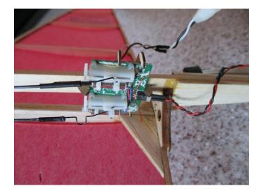
It uses a Spektrum brick for rudder and elevator with a single cell 200mAh LiPo battery.
