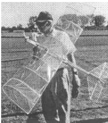
radio controlled model: Flying weight-10 oz.; Flying speed-seven mph; Wing Area-seven square feet; Wing loading - 1.4 oz per square foot. The picture of the model in the air was taken early Sunday morning in a very light breeze which the designer described as the practical limit for his model's ability to handle moving air. Quite an achievement!
