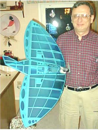
Rick Sawicki showed his Elipstik 460 ARF from Northeast Sailplane, 948 Hercules Dr., Suite 12, Colchester, VT 05446 – phone: 1-802-655-7700 – Web site: www.nesail.com. Rick added a pod to the bottom to carry various size battery packs and the R/C gear. It uses a S400 for power. It weighed 13.6 ounces with the original S280 power and now weighs 16.5 ounces with the S400 power.
