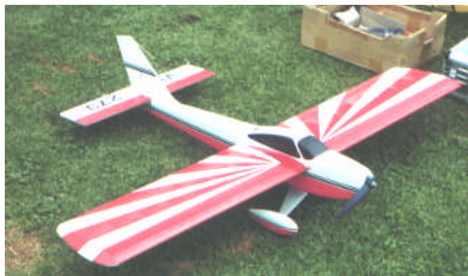
Australian produced kit "Electro Flash" - 12 cells - 64 oz. - fully aerobatic.
