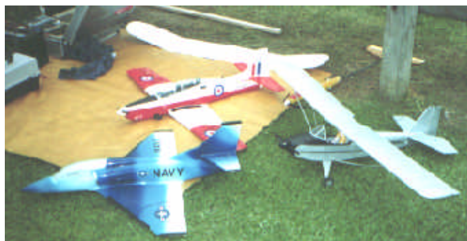
Ballistic "Skyhawk" 120 MPH 10-cell Plettenberg motor - all fibreglass - designed and built locally. 480 Powered Tucano - very fast & aerobatic Semi-scale Parasol - 540 powered
