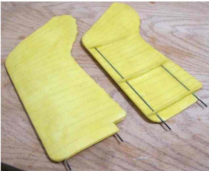
I did the "S" airfoil by hot-wiring some EPP, then trapped the 2mm Depron between. I put the foam assembly between two boards and weighted it. I preheated the oven to 250°F, turned it off and installed the weighted mold. When it is cooled, the Depron wing it holds its shape.
