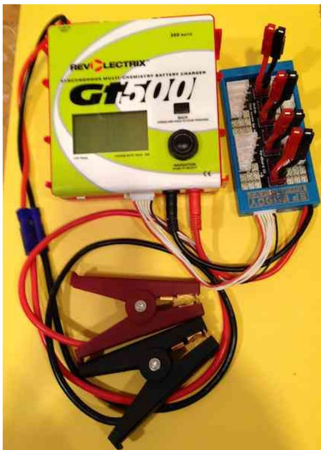
Battery types from the manual: “Lithium Polymer HV (1s to 8s balanced, 1s to 2s unbalanced), Lithium Polymer (1s to 8s balanced, 1s to 2s unbalanced) Lithium Ion (1s to 8s balanced, 1s to 2s unbalanced), Lithium Manganese (1s to 8s balanced, 1s to 2s unbalanced), A123 (LiFePO4) (1s to 8s balanced, 1s to 8s unbalanced), NiCd (1s to 21s), NiMH (1s to 21s), Lead Acid batteries (1s-12s Flooded, Gel, AGM, SLA)”.
