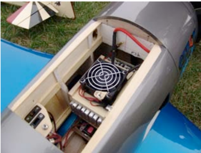
Battery cooling fan has been added over the Kokam 3200 mAh cells
