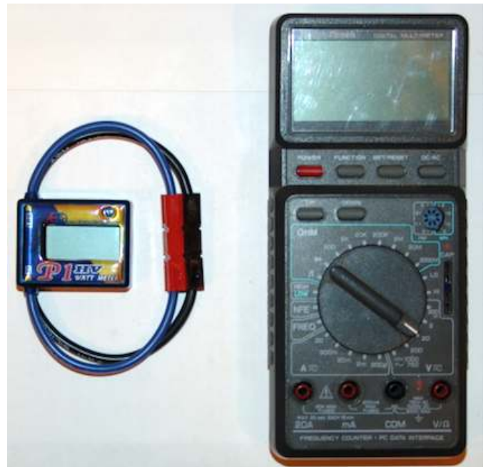
P1 HV with APP connectors added & Multimeter used for voltage calibration
