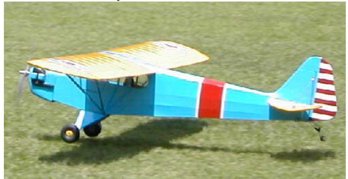
84" span, 8lb 20z, 20 x 2000mA NiMH cells and a MaxCim 13Y on 3.3:1 and a 15x8 APC-E - flies just like a Cub! The photo attached is her about to touch down - she's still a tad nose heavy, hence the near full up elevator as I flair to land. Superb kit, really simple conversion - I hardly did anything, beyond fitting a funny shaped 'engine' under the cowl and a larger 'gas tank' up front. Looking forward to *Ampeers* to come
