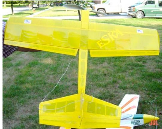
I have built all three of his kits to date. In addition to the fusion, he has the eSKA (electric simple kit airplane), and the Go-Go dancer. The eSKA is a 31" wing with a unique wing locking system, no bolts, and no rubber bands. It locks in solid, but will pop out if you meet terra firma nose down. The Go-Go is a 26" wing pusher, using CD-Rom motor that weighs 7 oz.
