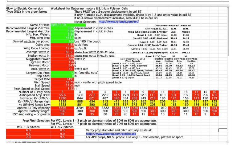
capacity that exceeded the pack that Mike wanted to use, which was a 3S 2200mAh. The spreadsheet suggested a capacity of 3700mAh for the 3S Li-Poly battery with decent flight times.
