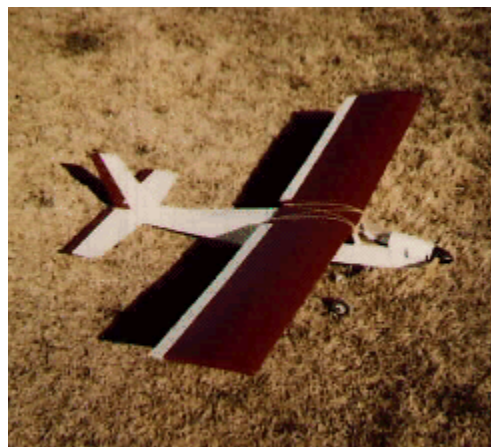
Specs for Richard's Mirage Mirage 550 - Span: 52" - Chord: 9.5" - Area: 494 ailerons added some area Weight: 46 oz Motor: Master Airscrew 05 geared 2.5:1 Prop: M.A. nylon 10 x 8
