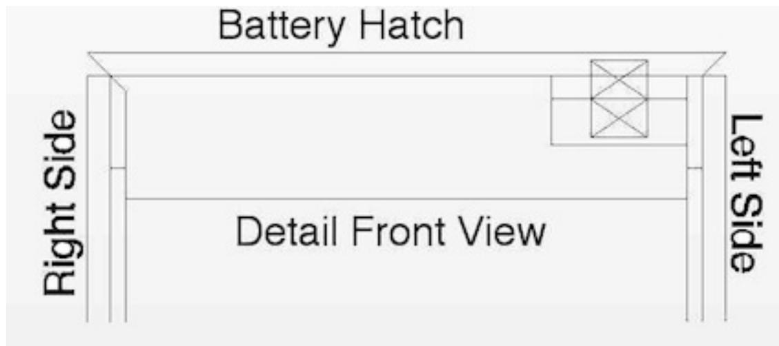
Sand the outside edges of the battery hatch to about a 45 degree angle on the fuselage sides. Sand, towards the inside, about a 45 degree angle on the right side of the battery hatch compartment fuselage side. The two angles on the right side allow using the covering as a hinge and on the left side a place to grab to open the hatch.
