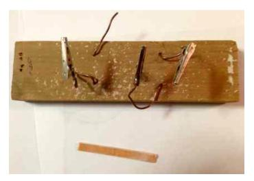
each other, though the wood. Run a nine inch length of wire through each hole until they are about equal. Solder on the clips. (put photo here)
