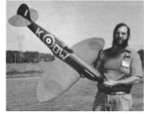
type and size. Slow-flying planes, such as, WWI or 1920 - 1930 light planes (Cub, Taylorcraft, etc.), use a 14 - 18 oz./sq. ft. wing loading, but for fighters and aerobatic types, a 20-25 oz./sq. ft. loading is more appropriate. Small planes (less than 400 sq. in.) should use the lower wing loadings
