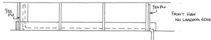
If you insist on using spruce, don't put the grain vertical, put it horizontal, so that the wire can't split the grain. The grain should run front to back on the wing and the hole for the wire goes up through this. This vertical piece is glued to the ply rib doubler on the inner end. That's where all the strength in the airplane is, at that one joint. The rest is going along only to prevent the wheel from wandering.
