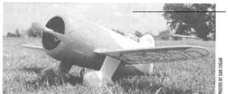
Even the infamous Gee Bee-R1 flies well as an electric, partly because of the near-scale diameter propeller.
