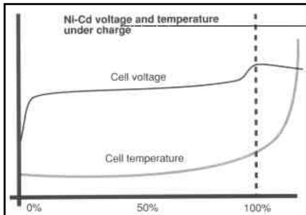
viable way to determine end of charge; in fact, virtually all rechargeable hand tools rely on this technique. The main drawback is that a temperature sensor must be in contact with the battery pack, which would mean a four-wire connection to the charger.
