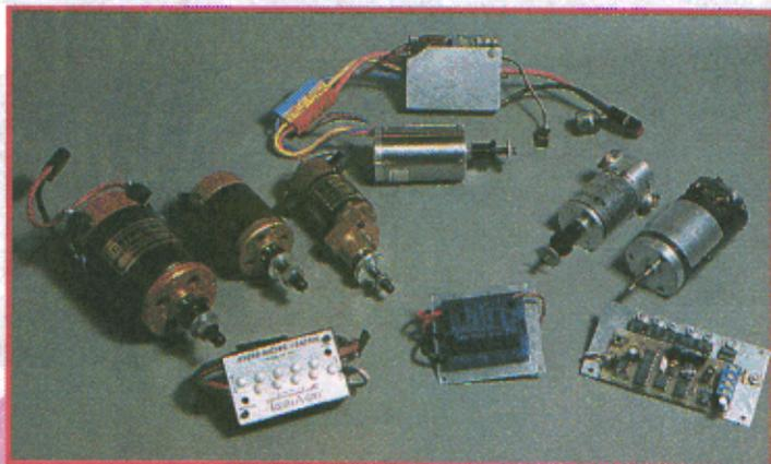
A collection of motors and speed controllers. Left to right: Astro Flight's 90, 25, geared 15, and the Keller 25 and 50. Front: the Astro 207, Jomar SM-4 and Jomar Maxcell speed controllers. Top: the Aveox "brushless" motor and special controller.
