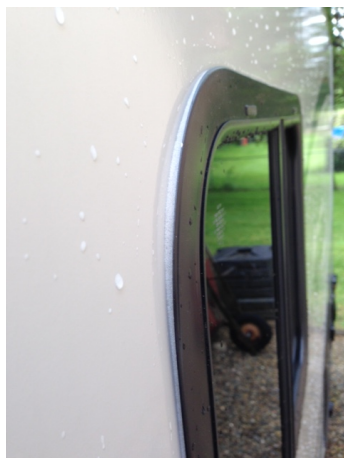
Photo 1: Kitchen Window, outside left taken this morning before I resealed it with Dynaflex 230.
