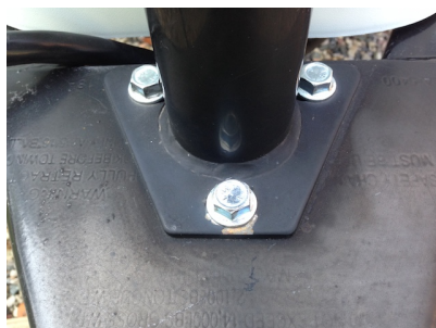
The tongue jack plate has rust on it.
