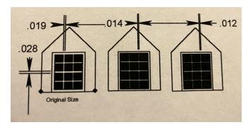
The CAD drawing, of the different size window muntins, was printed full size, with the printer set at "best", to print from the CAD program.
