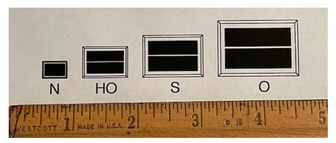
The four scaled windows, using 1:160 for N scale, 1:87 for HO, 1:64 for S, and 1:48 for O, were printed next to each other and a ruler laid on the print to give the prints scale.
