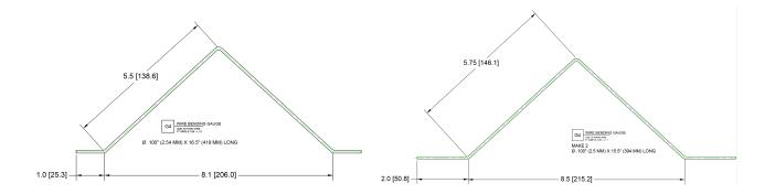
The only part that was modified, by Flite Test, was the landing gear wire, which they made slightly longer. That increased its height and width slightly, but they did not modify its forward position.
